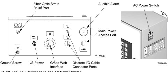
FIG. 13. EasyKey Connections and AC Power Switch
